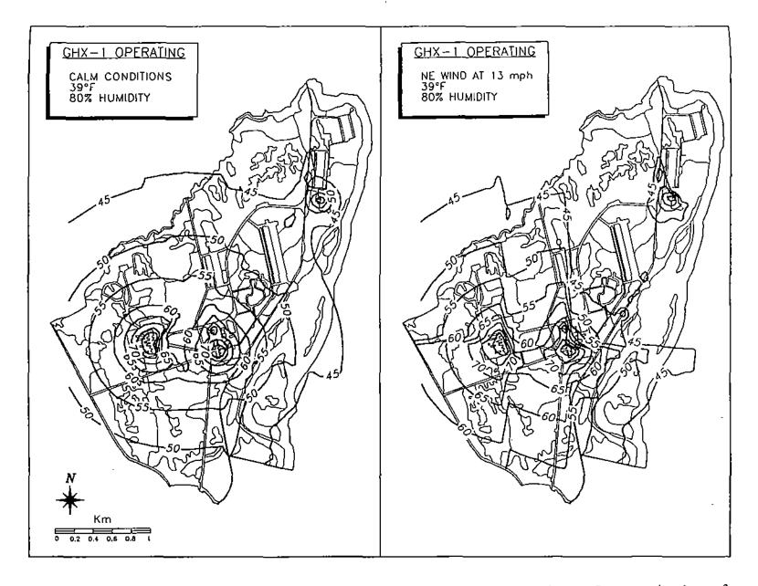
Predicted noise contours (5 dBA) around the CCP and CGF facilities during the first operational year for GHX-1 (1991) under calm and windy conditions in the GHX-1 study area, Prudhoe Bay, Alaska. Contours were modeled with the Outdoor Noise Prediction Program (McCraw 1992).
