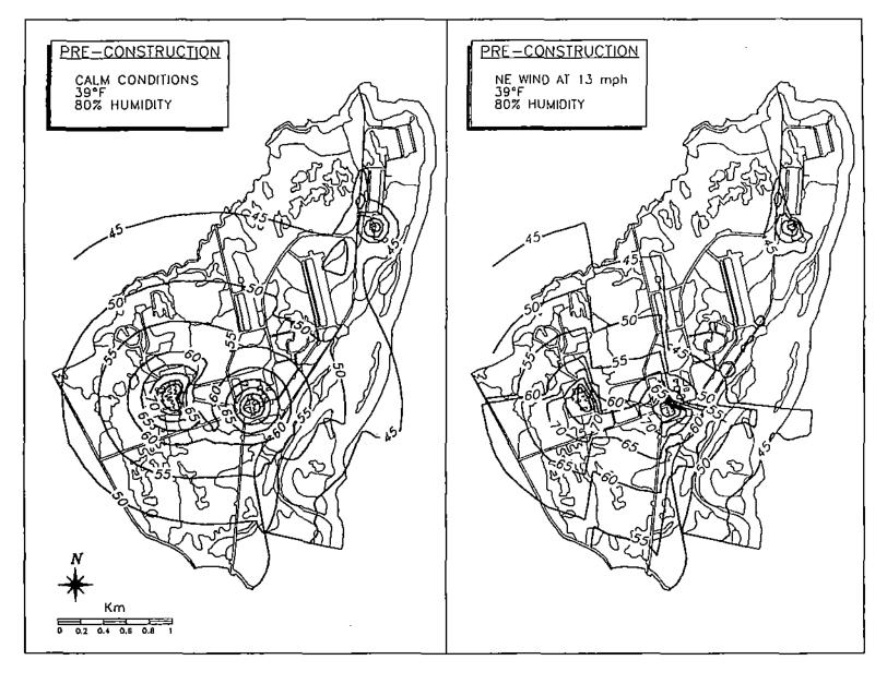
Figure 7. Predicted noise contours (5 dBA) around the CCP and CGF facilities during pre-construction (1989 and
