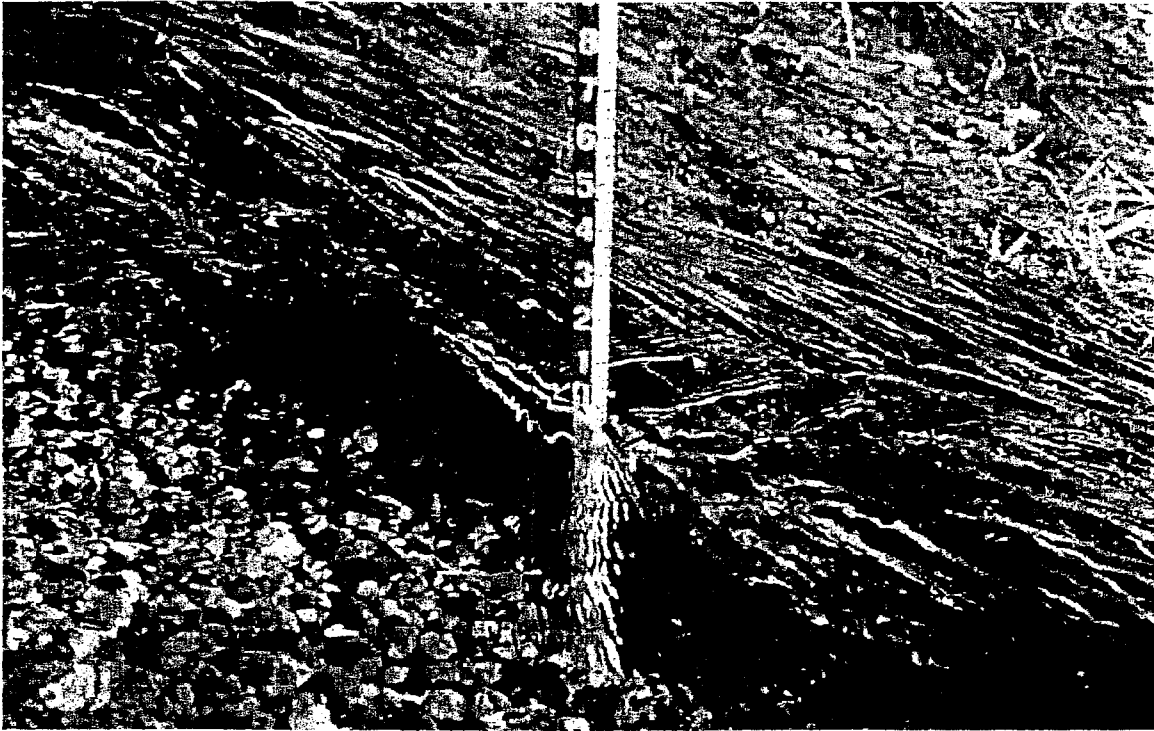
Photo C-5: Typical grass and gravel channel with medium flow. Note how the grass is laid down by the higher flow.
