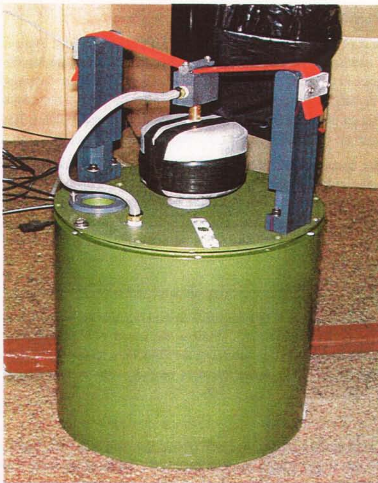
FIGURE 8.3. Photograph of a DASAR, as implemented in 2001, showing sensor suspension at top.
