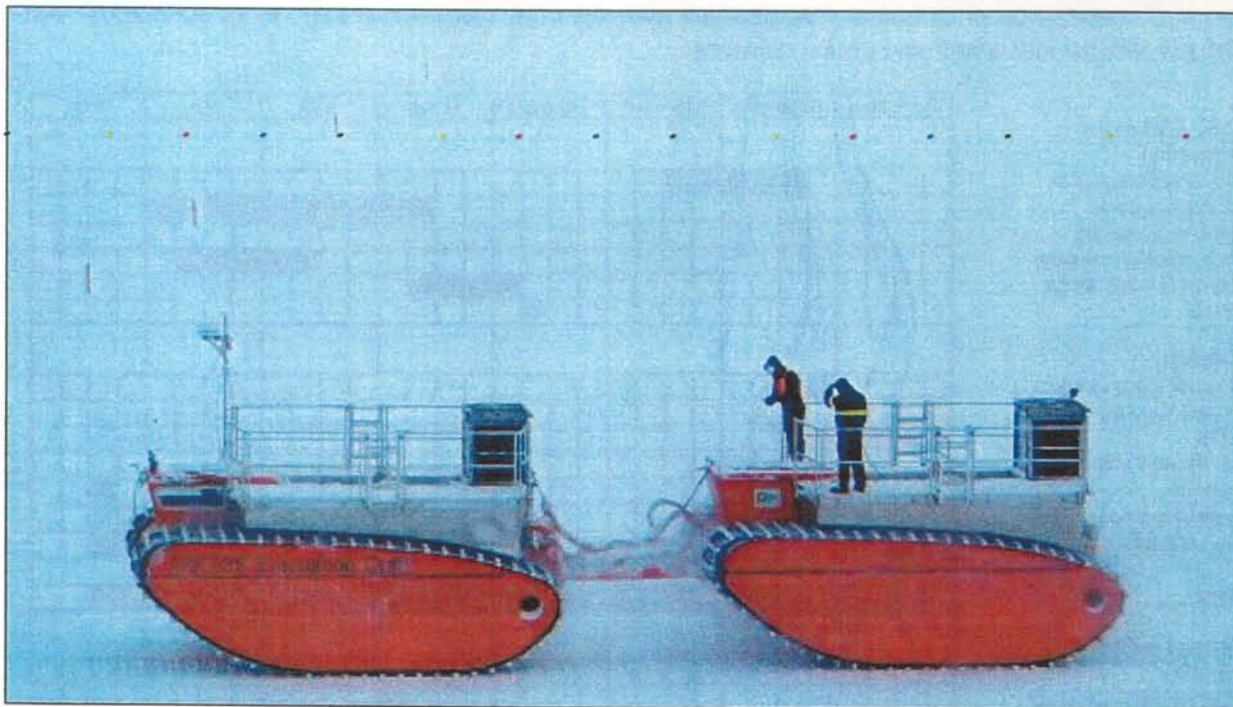
FIGURE 2.3. One of the two articulated ARKTOS evacuation craft that were used as the island emergency escape vehicles.
