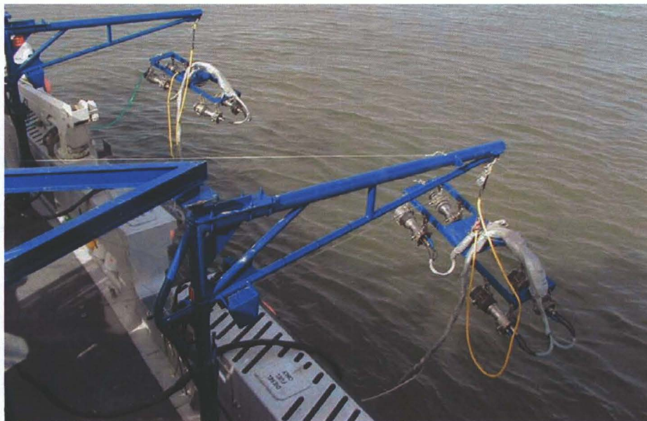
FIGURE 2.9. Starboard pair of 4-airgun clusters that formed half of the 320 in 3 airgun array deployed from the Peregrine in 2001 (photograph by J. Lawson, LGL). The square steel frames, suspended from the two davits kept the airguns positioned at the correct water depth and spaced precisely.
