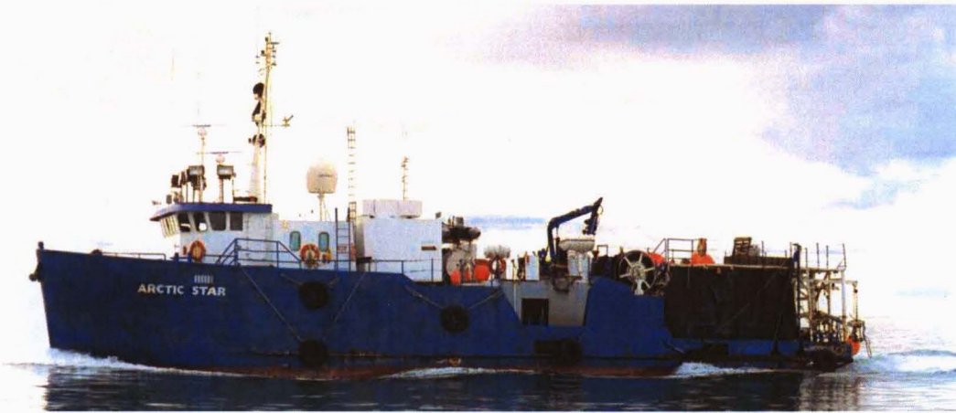
FIGURE 2.3. WesternGeco's larger source vessel, the R/V Arctic Star . This steel-hulled vessel was used to operate the 1210 in 3 airgun array (1999 photograph by W. Burgess, Greeneridge Sciences).
