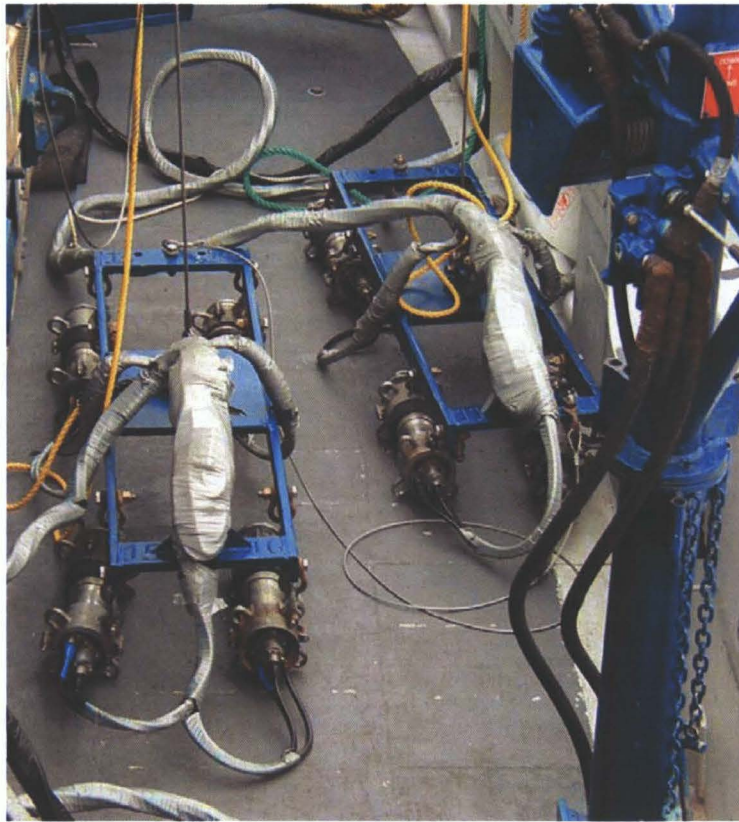
FIGURE 2.8. View of two 4-airgun clusters that formed half of the 320 in 3 airgun array deployed from the Peregrine in 2001 (photograph by J. Lawson, LGL). The gray tape covers and protects the high-pressure umbilical cables, which provided air pressure and firing control for each 40 in 3 airgun.
