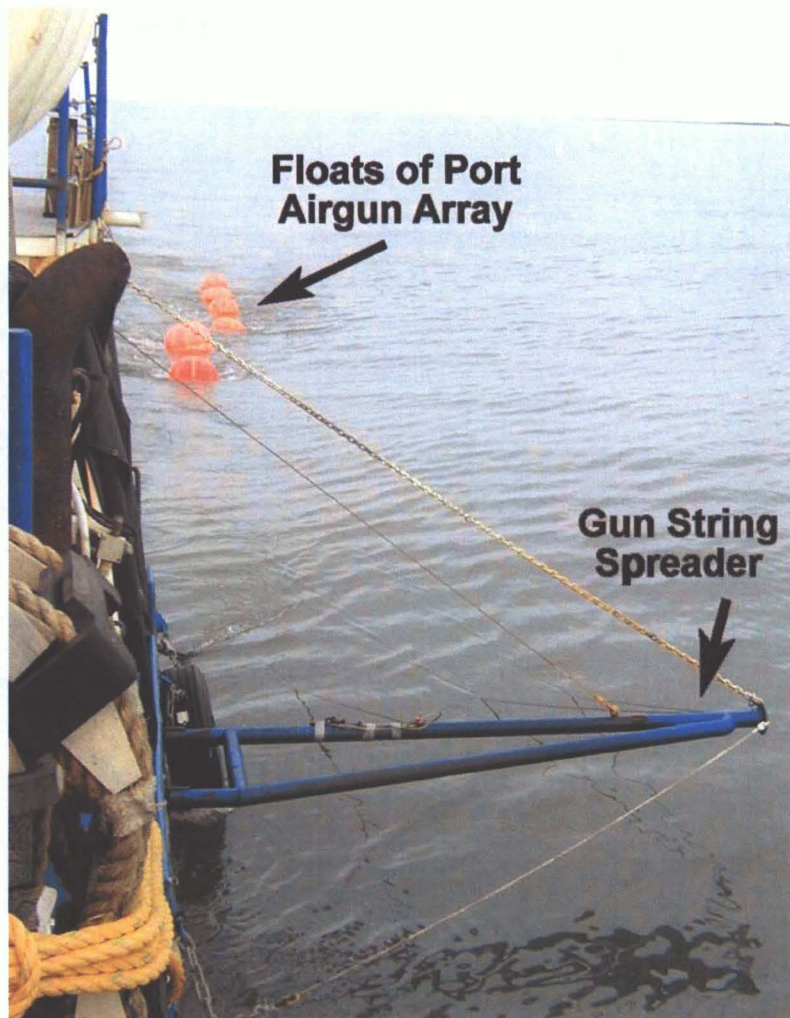
FIGURE 2.12. Horizontal spacing of the airguns was ensured by cable harnesses attached to two towing booms ("gun string spreaders"), which extended out from either side of the R/V Arctic Star during seismic operations. The floats of the port side of the airgun array can be seen in the water astern of the vessel (photograph by J. Lawson, LGL).
