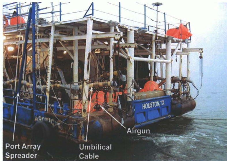
Figure 2.10. The 1210 in 3 airgun array stowed aboard the R/V Arctic Star (photograph by J. Lawson, LGL). The airgun umbilicals can be seen hung from chain supports, as well as the array floats and the airguns themselves.
