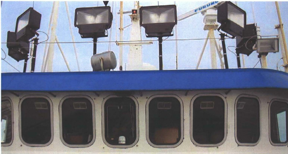
FIGURE 2.4. Six broad-beam, 1000-Watt floodlights above the bridge of the R/V Arctic Star (1999 photograph by J. Lawson, LGL).
