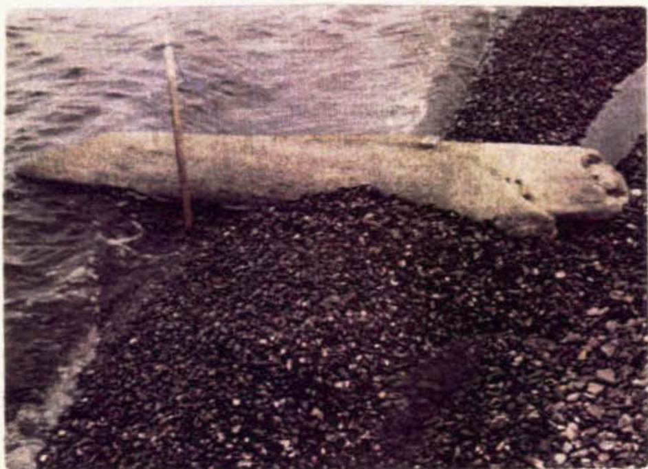
PHOTO 30. SEDIMENT BLOCKAGE AT BARRIER AFTER ONE HOUR, LOCATED ON GRAVEL SPIT NEAR TRANSECT #27
