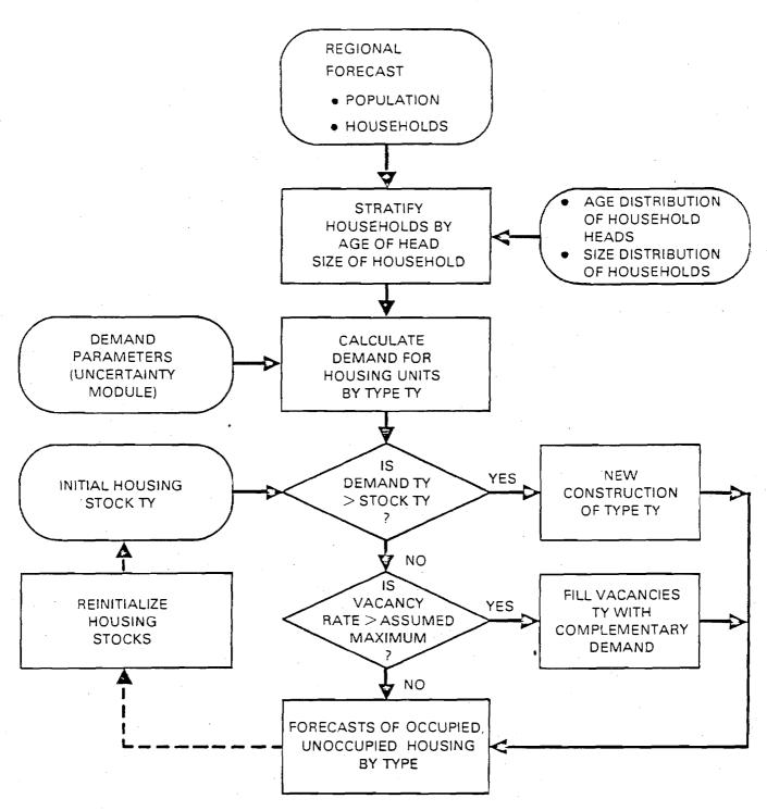
FIGURE 4.1. RED Housing Module
