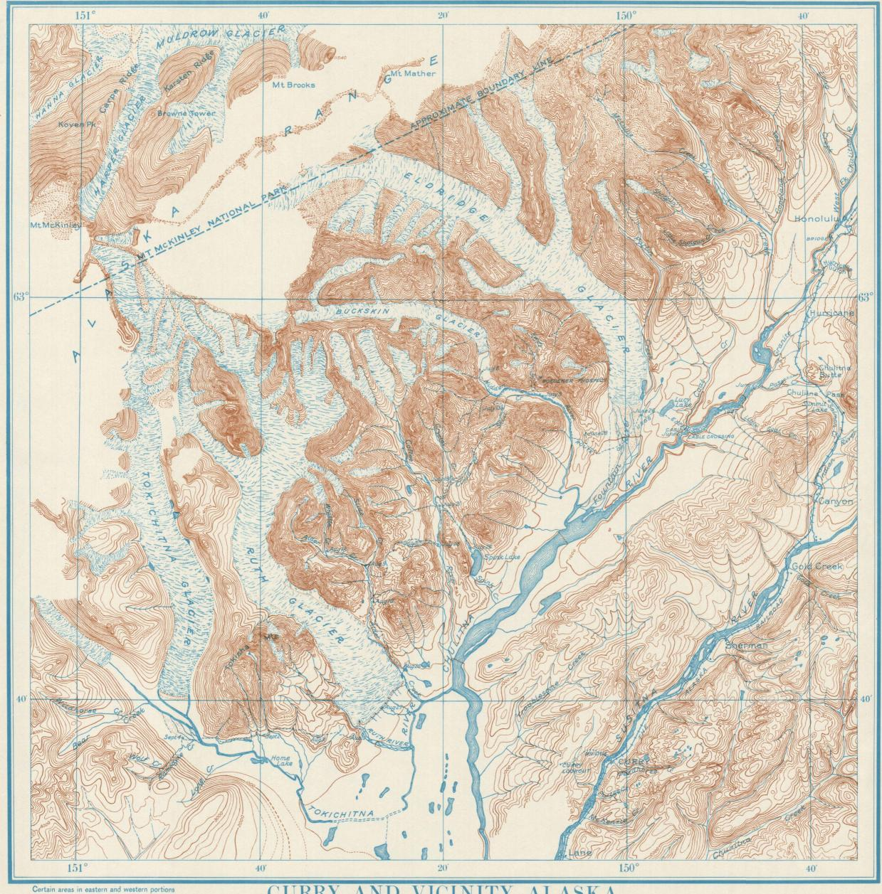
Certain areas in eastern and western portions from earlier U. S. Geological Survey maps. Geodetic position based upon data by U. S. Coast and Geodetic Survey. Areas not surveyed, in detail indicated by broken lines Surveyed in 1932
