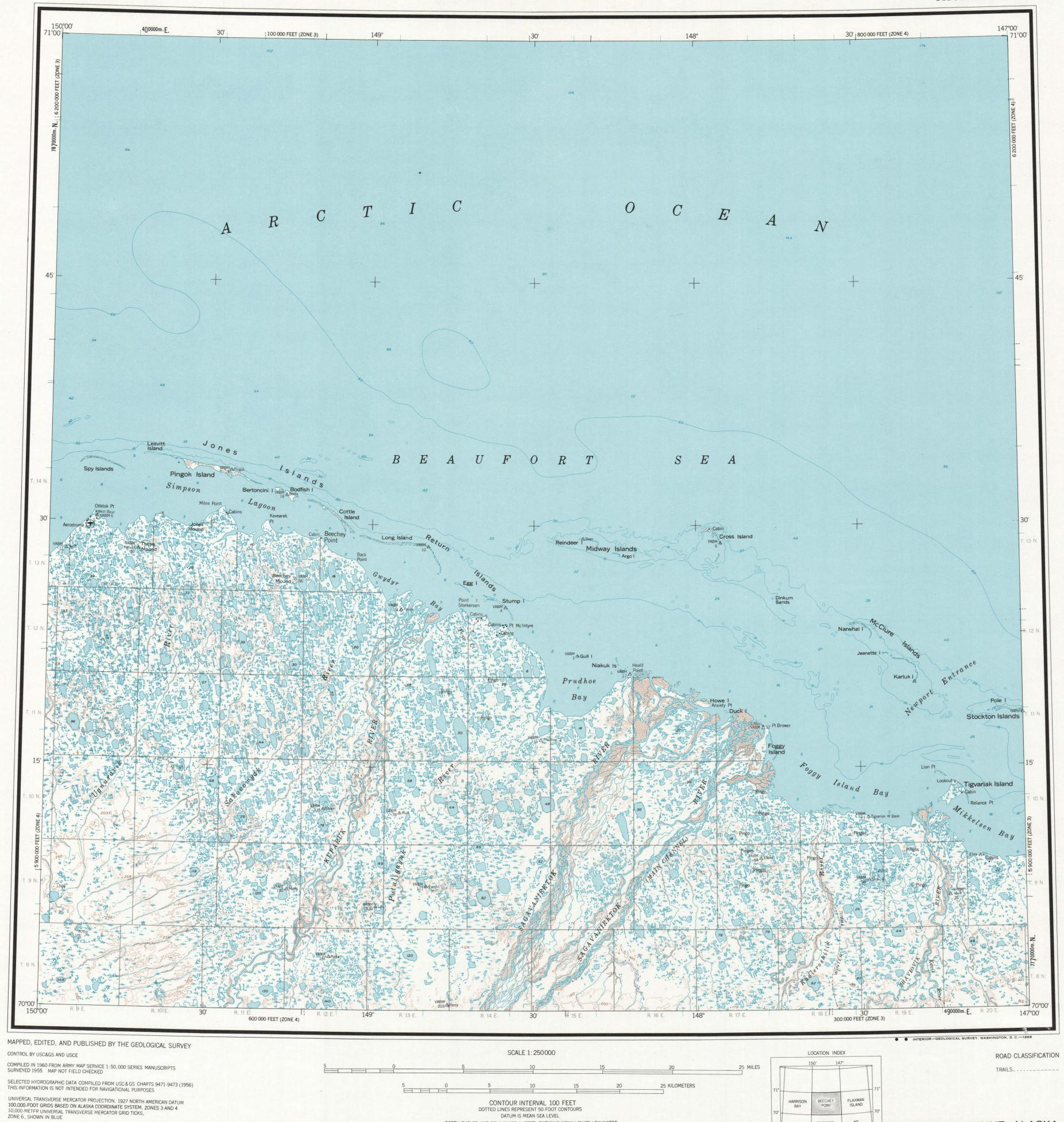
DEPTH CURVES AND SOUNDINGS IN FEET. DATUM IS MEAN LOWER LOW WATER SHORELINE SHOWN REPRESENTS THE APPROXIMATE LINE OF MEAN HIGH WATER 1955 MAGNETIC DECLINATION AT SOUTH EDGE OF SHEET VARIES FROM 31°00' TO 33°00' EAST THIS MAP IS AVAILABLE IN BOTH SHADED RELIEF AND CONTOUR EDITIONS
