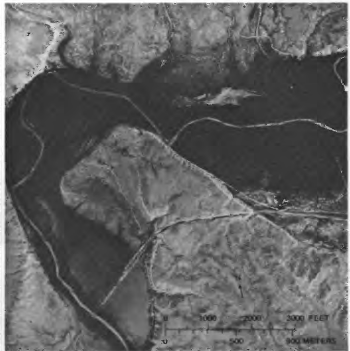
FIGURE 9.—Aerial view of conditions of a part of the Gila River channel above the San Carlos River in June 1962. Flow in the river is from upper right to lower left. The channel is continuous, but a comparison of this photograph with figure 8 indicates that the width has been reduced and the riverbed has been considerably elevated. Extensive ephemeral off-channel ponds are shown in the vicinity of the abandoned railroad crossing.
