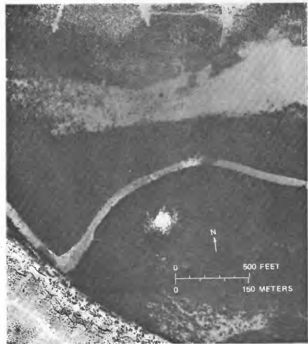
FIGURE 16.—Aerial view of channel plugging in the Gila River on July 22, 1964. Flow is from right to left.
