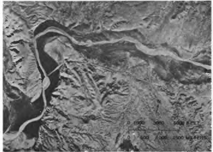
FIGURE 8.—Aerial view of channel conditions of the Gila River upstream from the San Carlos River in 1935-7 years after the completion of Coolidge Dam. The upstream end of the reservoir pool is shown in the lower left. The Gila River flood plain shown in the photograph had been inundated by the reservoir pool during the period 1929-35. Soil Conservation Service photograph.
