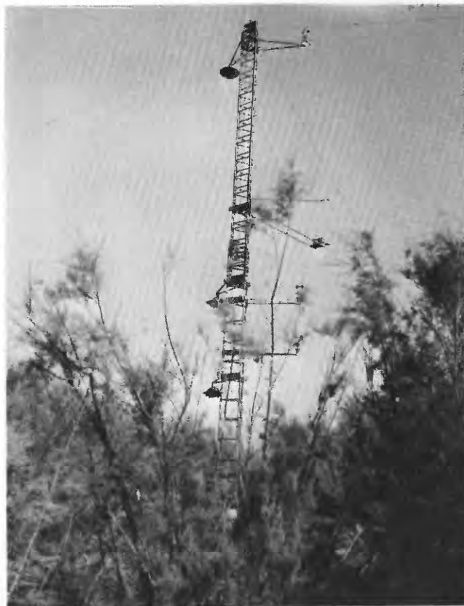
FIGURE 10.—Energy-budget station in operation at section 19.
