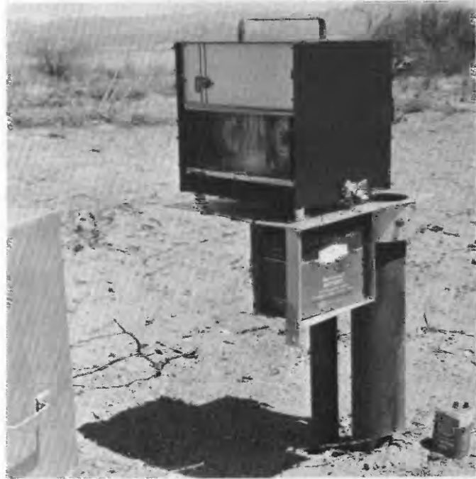
FIGURE 7.—Water-level observation well, showing installation of digital recorder.
