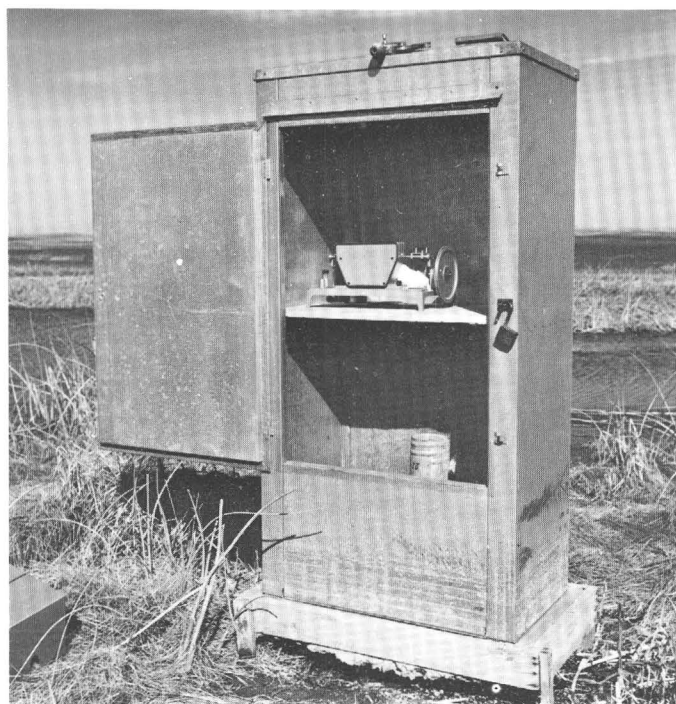
FIGURE 13.—Type-F recorder in shelter at well 22N, pothole C1.
