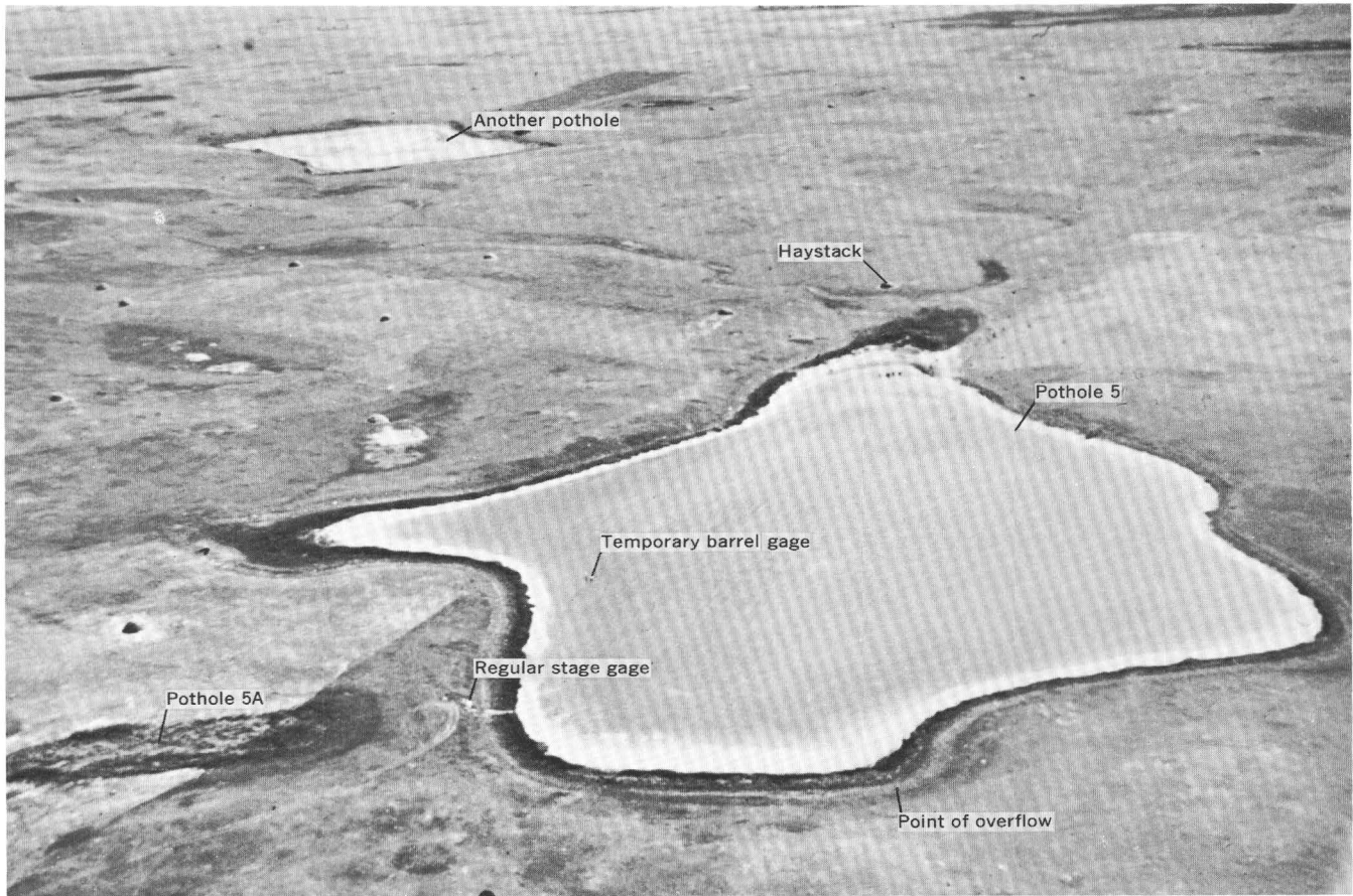
FIGURE 28.—Potholes 5 and 5A near Forbes. Photograph by W. P. Sebens, Executive Secretary, North Dakota State Soil Conservation Committee, September 16, 1961.
