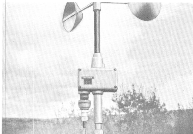
FIGURE 9.—Totalizing anemometer. Photograph by Roger Pewé, September 13, 1965.
