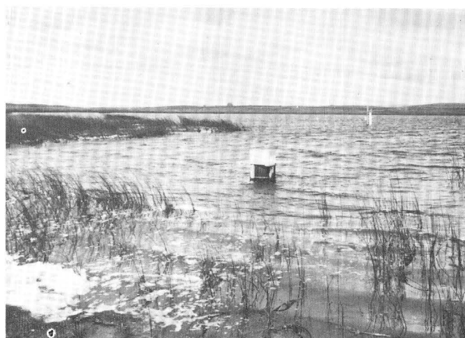
FIGURE 32.—Pothole C1, showing instruments. Note wave action that made difficult the precise determination of pond level.
