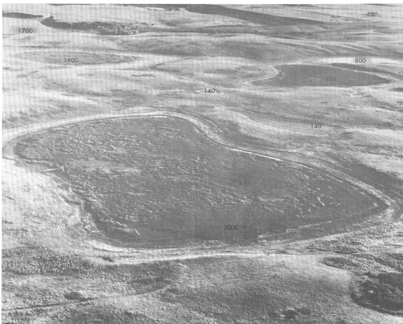
FIGURE 26.—Aerial view of pothole 4, viewed toward the south-southwest. Numbers on potholes indicate specific conductances, in micromhos per centimeter, measured June 11, 1963. Photograph by W. P. Sebens, September 1961.
