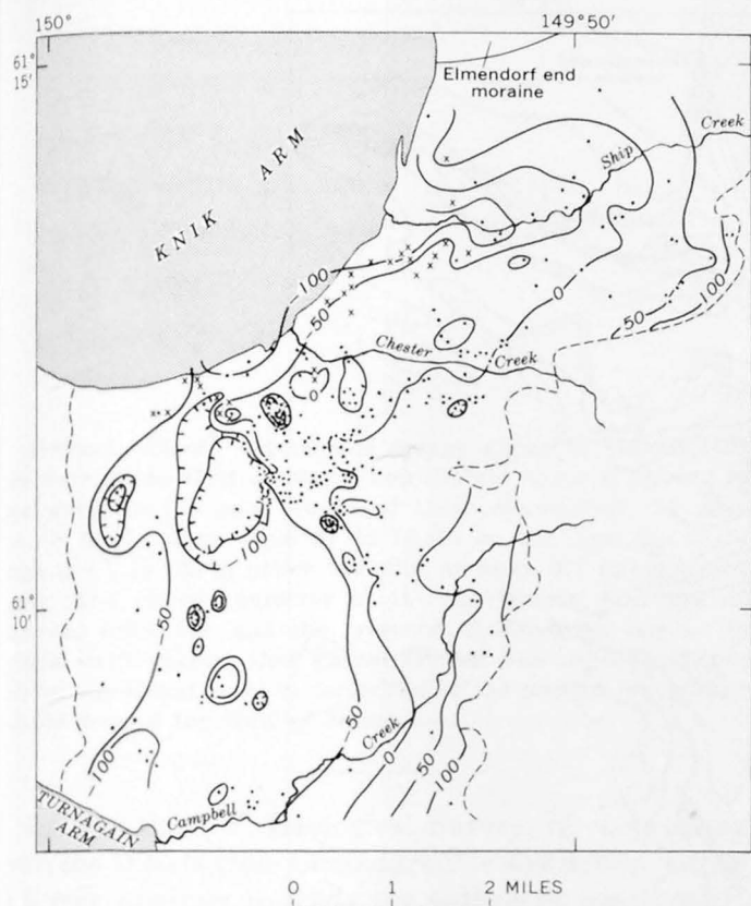
FIGURE 5.—Contour map of the base (unconformity) of the Bootlegger Cove Clay in part of the Anchorage area. Datum is mean sea level; contour interval, 50 feet. Dots show location of wells from which data were obtained for drawing contour lines. Dashed lines show inferred boundaries of the clay.
