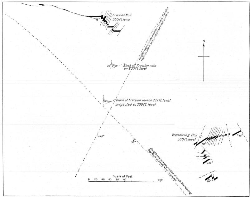
HORIZONTAL PLAN OF VEINS AND FAULTS IN WANDERING BOY AND FRACTION 300-FOOT LEVELS, TOGETHER WITH PROJECTED POSITION OF THE MAIN FRACTION AND WANDERING BOY FAULTS AT THIS LEVEL.
