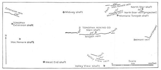
FIG. 70.—Map showing principal earlier andesite veins now developed undergound, within the main productive area: shown on the horizontal plane of the Mizpah 500-foot level.
