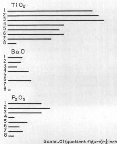
FIG.74.—Diagram showing relative proportions of the less common elements in the various stages of alteration of the earlier andesite.
