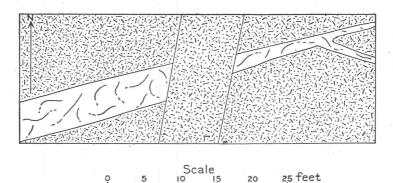
FIG. 23.—Horizontal sketch plan of portion of the Mizpah vein in stopes east of Lease 52, about 70 feet from surface, showing probable compensating faulting.
