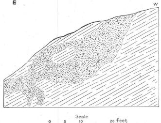
FIG. 8.—Vertical sketch section taken at a point on the east side of Butler Mountain, 100 feet below the contact of Butler dacite and tuff, showing dike of light-brown, semi-consolidated sand, of volcanic origin, containing angular fragments of dacite glass, intrusive into Siebert tuffs (lake beds).
