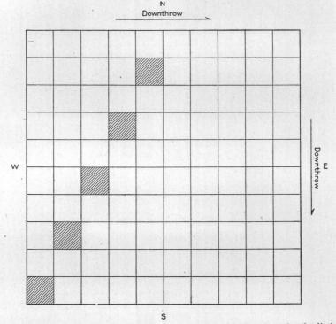
FIG. 54.—Diagram showing the effect of cross-faults when the faults of one system have twice the displacement of those of the other system. Here the north-south faults have double the displacements of the east-west ones. The shaded blocks are blocks of equal displacement.
