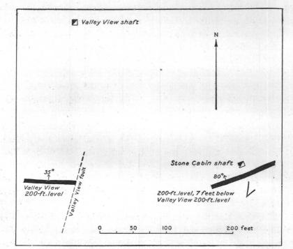
FIG. 33.—Horizontal plan of veins in Valley View and Stone Cabin workings on the plane of the Mizpah 200-foot level, to show the probable connection between the chief veins on the two sides of the Valley View fault.
