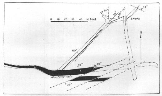
FIG. 60.—Horizontal plan snowing veins and faults on the 460-foot level of the Montana Tonopah.
