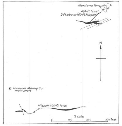
FIG. 62.-Horizontal plan showing relations of the Mizpah and Montana veins on the 400-foot level of the Mizpah.
