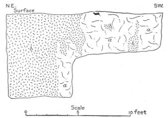
FIG. 72.—Vertical sketch section of shallow trench just north of Belmont shaft, showing contact of the Oddie rhyolite intrusion with the later and esite. a=Oddie rhyolite; b=later and esite.
