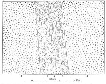
FIG. 15.—Vertical cross section of outcropping fissure vein, 20 feet west of section shown in fig. 14. 1. Calcite with angular rhyolite fragments; 2, quartz; 3, white rhyolite.
