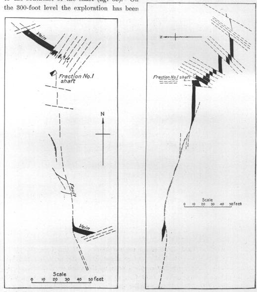
FIG. 35.—Horizontal plan of vein and faults on the 23/foot level, Fraction No. 1 workings.
