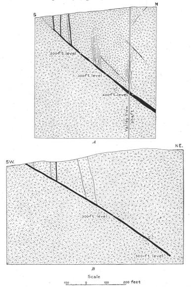
FIG. 29.—Cross sections of the Valley View vein. A, Through the Valley View shaft. B, Cross section of Valley View vein taken a short distance (averaging 200 feet) west of section A.
