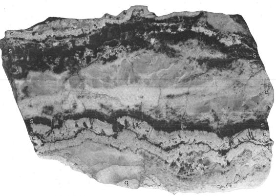
FRAGMENT OF MONTANA VEIN, ACTUAL SIZE, SHOWING CRUSTIFICATION.  $\label{eq:q} q= quartz, \ c= carbonates, \ s= rich \ black \ sulphides.$
