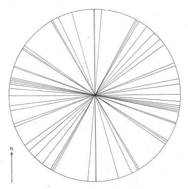
FIG. 34.—Plotting of the strike of the faults in the Fraction workings.
