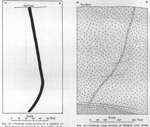
Mizpah vein as exposed in the Oddie shaft, showing reversed dip near the surface.
