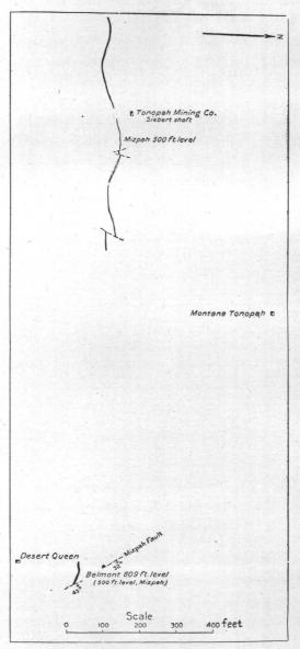
FIG. 26.—Horizontal plan of mine workings, showing the relation of the vein in the Desert Queen workings to that on the corresponding level of the Mizpah mine.
