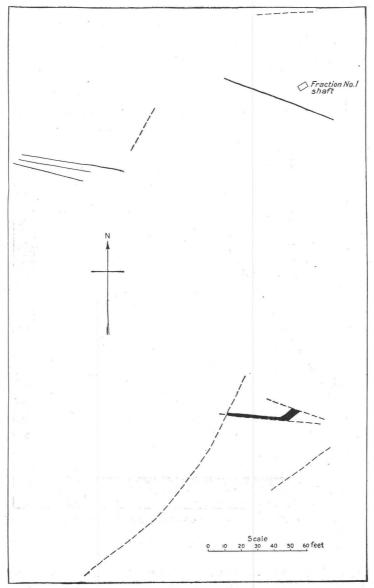
FIG. 37.—Horizontal plan showing veins and faults on the 400-foot level, Fraction No. 1 workings.
