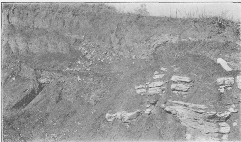
A. PINNACLE OF PLATTIN LIMESTONE OVERLAIN BY A BED OF MANGANESE-BEARING CLAY AND THIS IN TURN BY NON MANGANESE-BEARING CLAY WITH CHERT FRAGMENTS, IN NORTH CUT AT POLK SOUTHARD MINE.
