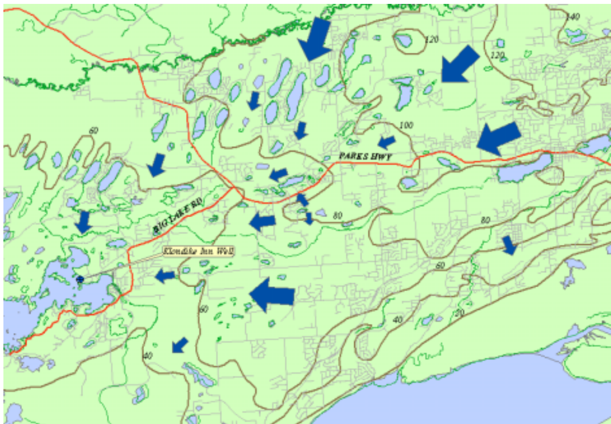
Figure 2. Map showing regional ground-water flow in Matanuska-Susitna Valley. (Jokela, Munter and Evans, 1991)
