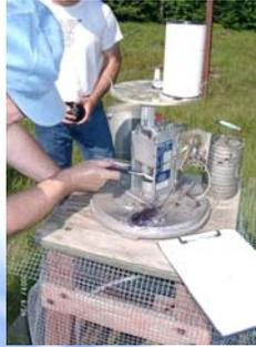
**If necessary, add oil, clean dash pot and replace oil. Or in some cases fill with oil as some new gages have been operating without.**
