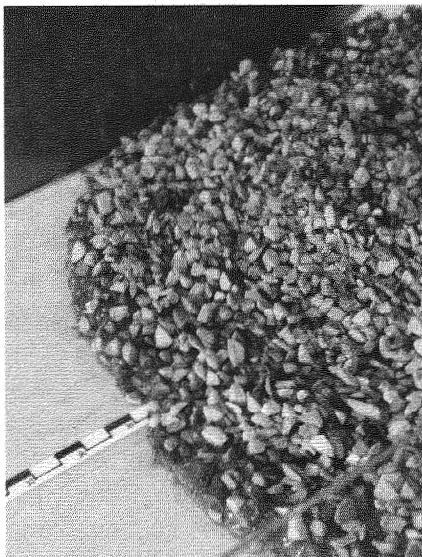
Figure 2. Slightly mixed mass comprised of sand and gravel heterogeneously covered by a brittle layer of dry gravel: Distinctive ridges appear, single gravel particles are dislocated, viscous material is pushed from underneath to the surface and amplitude of ridges increases (exp. no 18).
