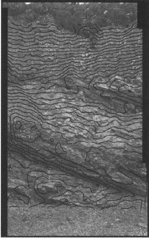
Figure 2. Contour lines of 5 cm equidistance draped over an ortho-photo. The size of the model area is 3.3 by 2.8 meters (height and width respectively).
