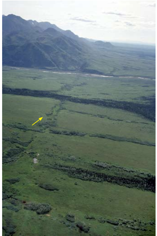
▲ Figure 14. Trace of the Denali-Farewell Fault (arrow) cross-cutting Quaternary alluvium on the north side of the Alaska Range near Farewell. View to the west.
