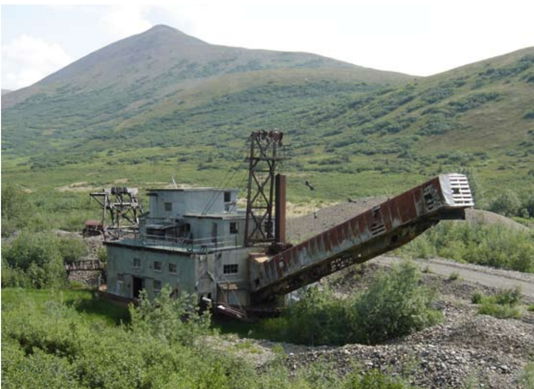
Figure 27. Inactive bucket-line dredge on upper Bear Creek, a tributary of the Tuluksak River. Dredges operated on this drainage almost continuously from 1925 to 1988.
