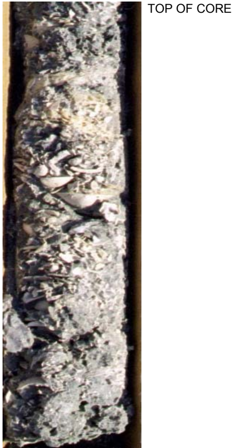
Figure 35. Marine sediments of late Miocene age from the Eastover Formation in the North core, borehole local number 59H 4, in Mathews County, Virginia (borehole location shown on plate 1). Core diameter is approximately 2 inches, and interval is between approximately 91 and 92 feet below land surface. Abundantly fossiliferous, medium- to coarse-grained sand constitutes lower part of the Yorktown-Eastover aquifer. Similarly fossiliferous part of the Yorktown Formation of early to late Pliocene age constitutes most of the remaining part of the Yorktown-Eastover aquifer. Fossil shells of the Eastover Formation are distinguished from those of the Yorktown Formation by inclusion of the distinctly pearly lustered mollusk Isognomon maxillata .
