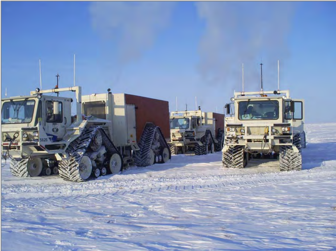
Example of vibroseis trucks conducting a seismic survey.
