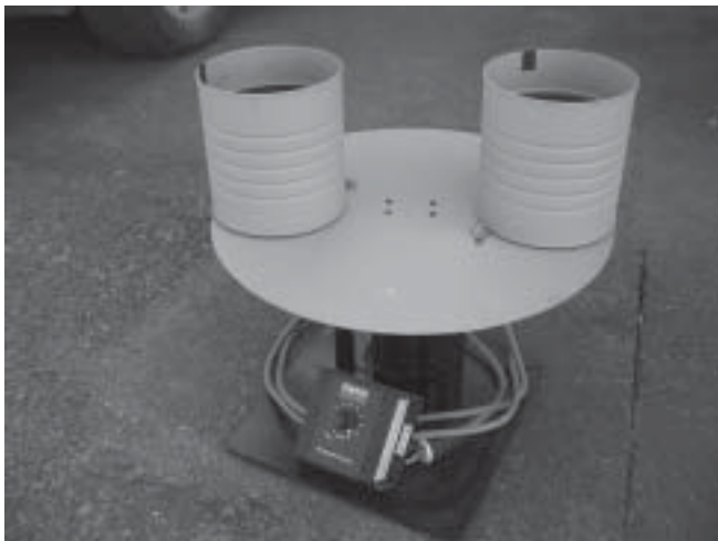
Figure 4 —This whitebark pine seed scarifier is being evaluated at the USDA Forest Service Coeur d'Alene Nursery, Idaho.
