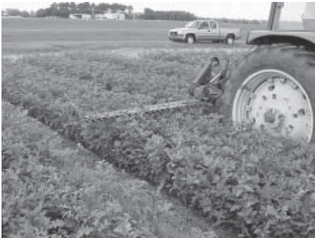
Figure 5 —Sickle-bar clippers used to manage shoot growth in bareroot seedling beds.
