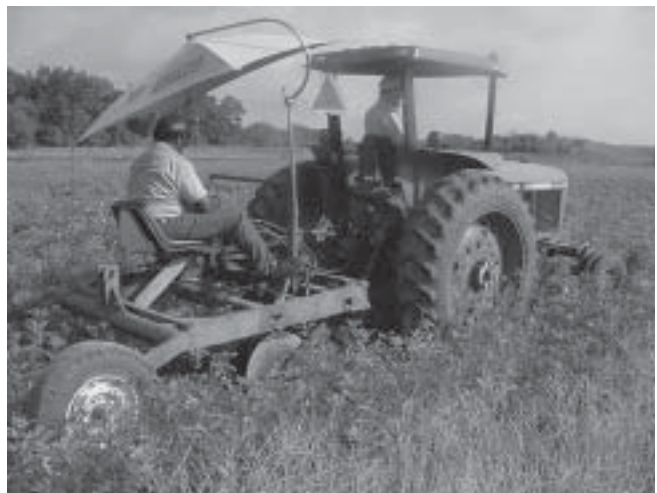
Figure 3 —Rolling coulter blades used to manage lateral roots in bareroot seedling beds.
